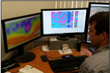
This data is then used to convert the EM38 map into a zone map, with potential high and low rate strip areas indicated that pass across all zones. Maps are produced and also placed on a GPS tablet to assist in ground truthing the paddocks with the farmers.
