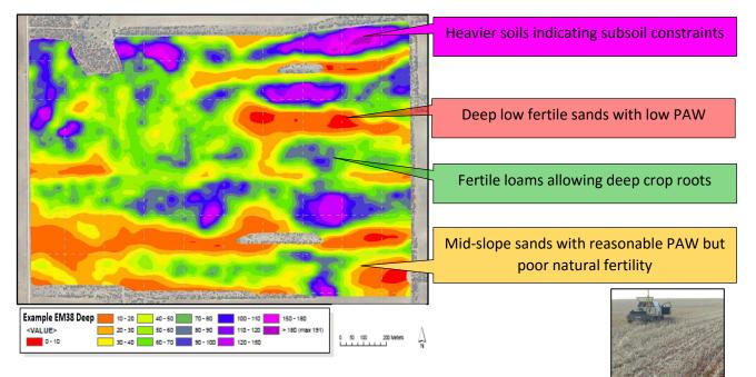
2. These EM38 maps are used to target 5 key soil testing areas to ground test the map information. The deep soil testing is done at 4 depths to 80cm, and analysed for texture, fertility, moisture content and subsoil constraints.
